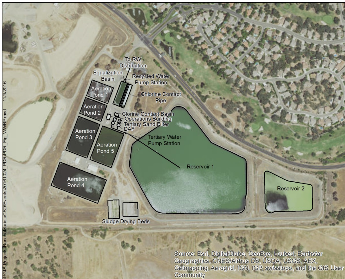
Figure 10. Existing WWTF and WWRP
